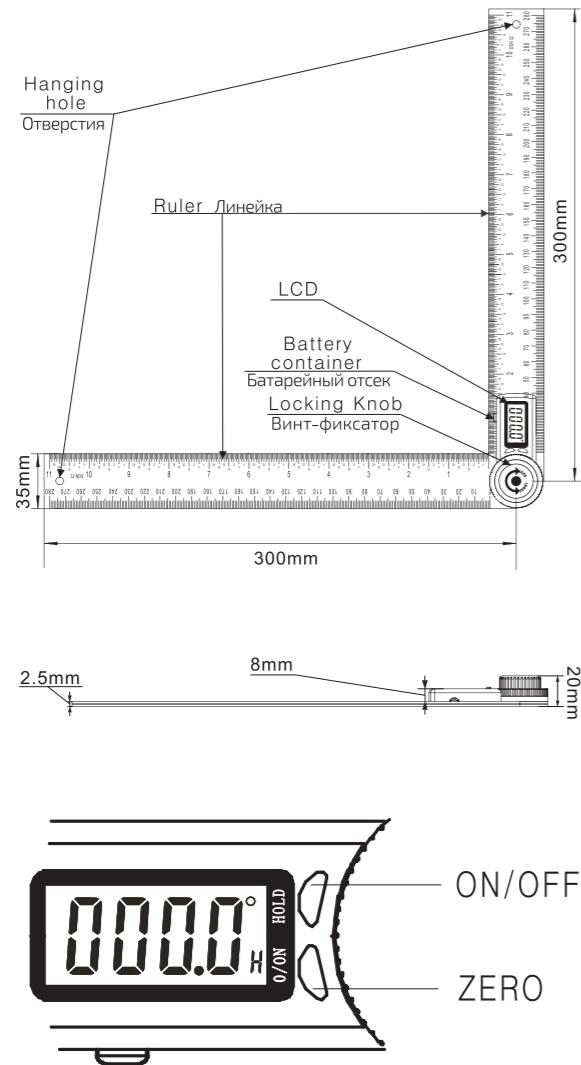
**ON/OFF** Short press ON/OFF to turn on the device. Short press ON/OFF to shut off the LCD. Long press ON/OFF for more than 3 seconds to shut off the whole system. Automatically shut off function in 6 min. Move the scale to turn on the device when at off LCD status.
